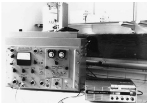
Figure 2: The Kay Elemetrics Spectrum Analyser 7029A was the sonograph model in use at the Laboratoire d'Acoustique Musicale in the 1960s and 1970s.
