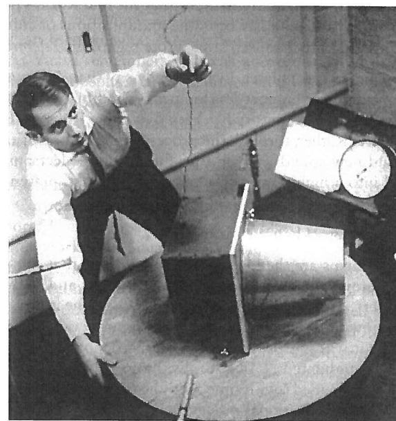
Karlheinz Stockhausen at the rotation table in the WDR Studio in 1958. This photo shows Stockhausen’s method at the time for achieving sound distribution in a concert hall. As the table is turned, the loudspeaker on it projects a sound in different directions. The sound is picked up at slightly different times by four directional microphones, placed at different positions around the table, and the signal from each microphone is recorded on one track of a four-track tape. When the tape is played back in a concert hall, the signal from each track is routed through a different loudspeaker. Photo courtesy Stockhausen-Verlag.
