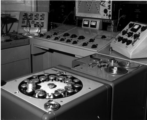
Figure 1. A view of the studio in 1953. The two machines on the lower side of the image are the two phonogènes : the chromatic phonogène and the sliding phonogène . (copyright GRM).
